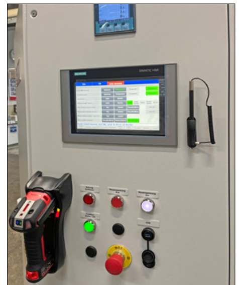
DEUTROFLUX MEMORY CONNECT parameter memory with additional handheld scanner for component identification
