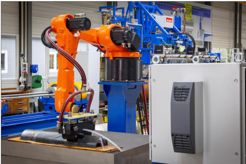
ECHOGRAPH SNHF PAUT system overview: robot arm with probe holder, phased array electronics cabinet and calibration station
