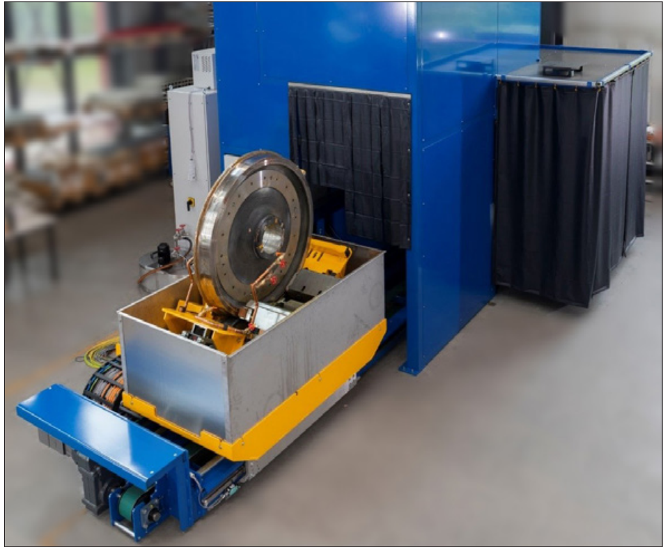
Loading carriage with customised test wheel and artificial flaws for process validation during pre-acceptance
