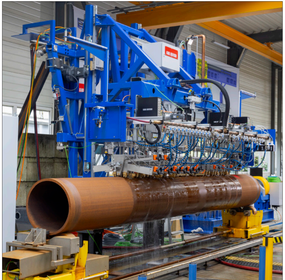
ECHOGRAPH SNUL: Height-adjustable trolley with test carriage and testing systems lowered onto the test pipe for application tests by means of the in-house roller conveyor
