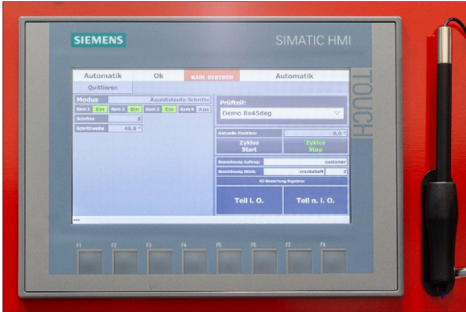
Figure 6: SIMATIC HMI touchscreen for controlling the test sequence
