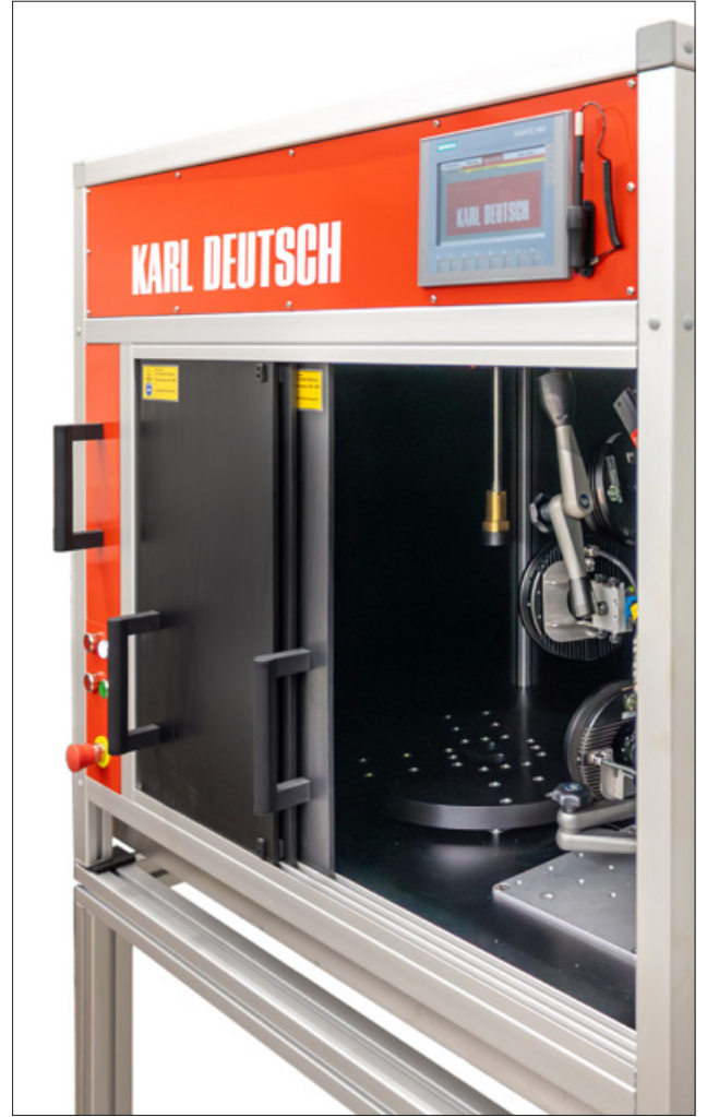
View of a CRACKVIEW AI test station with turntable for holding components, UV lights and camera
