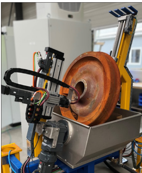
The UT test cycle for the largest diameter takes less than 60 seconds (without robotics).
