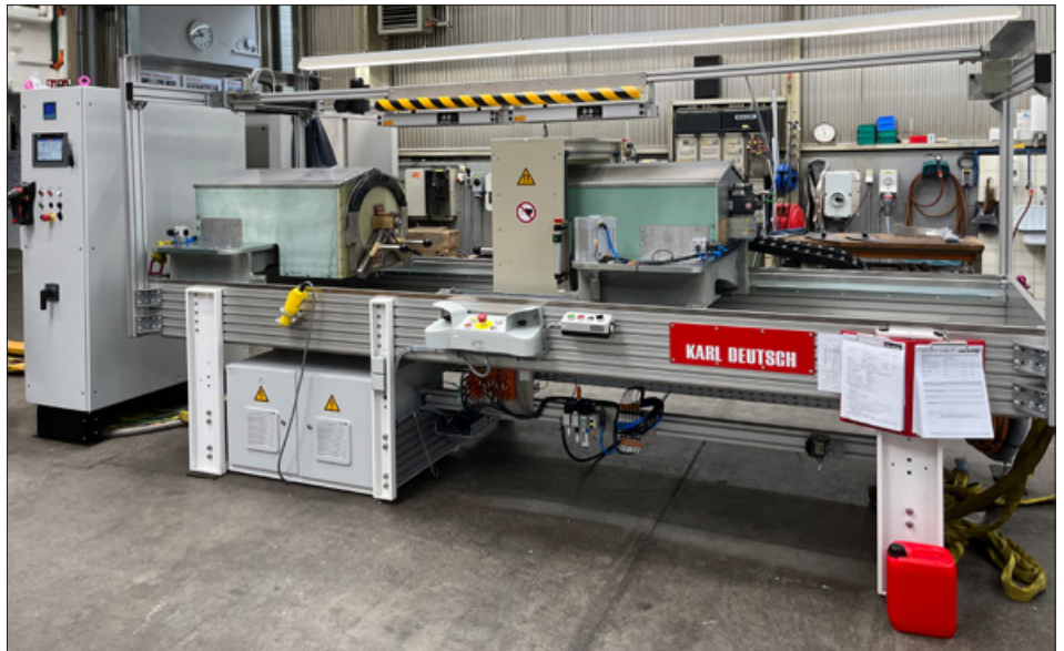
General view of the DEUTROFLUX UWS 1500 SPECIAL testing system incl. pneumatic UV lamp holder for better crane loadability
