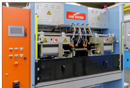
Front view of DEUTROMAT DAS-1U: magnetisation station with two exchangeable mandrels, each with internal flushing
