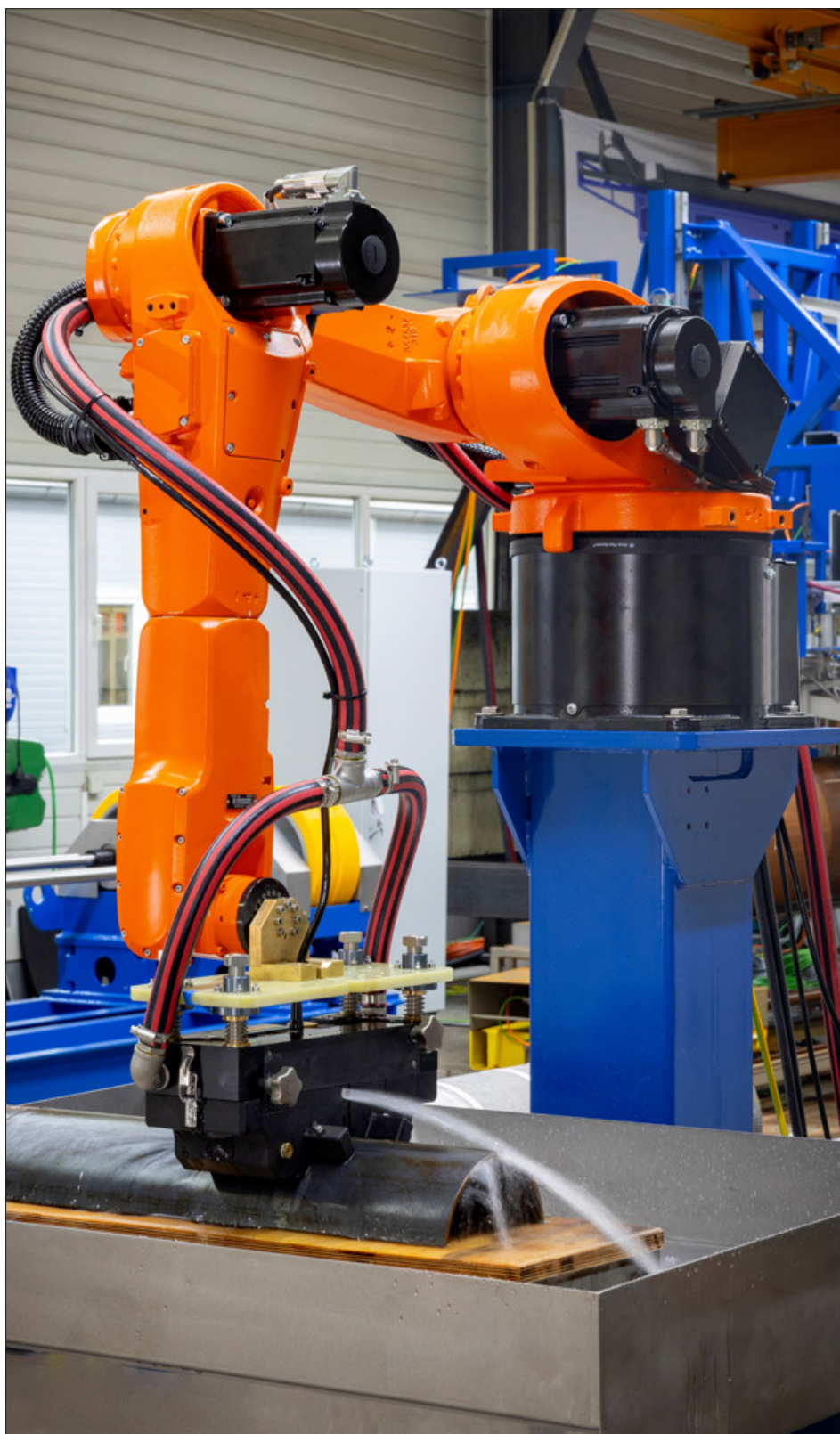
ECHOGRAPH SNHF PAUT with dynamic reference measurement on the pipe half-shell with artificial flaws during internal commissioning in our Works 2
